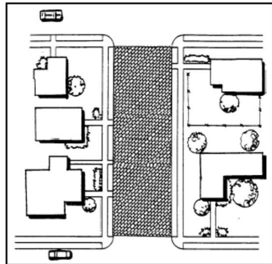
**Raised intersections** are speed tables covering entire intersections, with ramps on all approaches using brick or other textured materials on the flat section. The textured surface provides a visual cue to the driver to slow down. These intersections rise to sidewalk level, or slightly below to provide a "lip" for the visually impaired. They make entire intersections into pedestrian territory.
