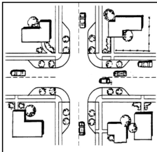
**Neckdowns** utilize curb extensions at intersections to reduce roadway width thereby shortening pedestrian crossing distance and enhancing pedestrian visibility. Neckdowns are the most common type of street narrowing. Issues to consider with neckdowns include drainage structure relocation, parking or truck movements, landscaping, and location of bus stops.
