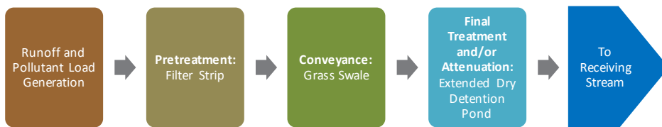
Figure 3: Example of a Stormwater Treatment Train
